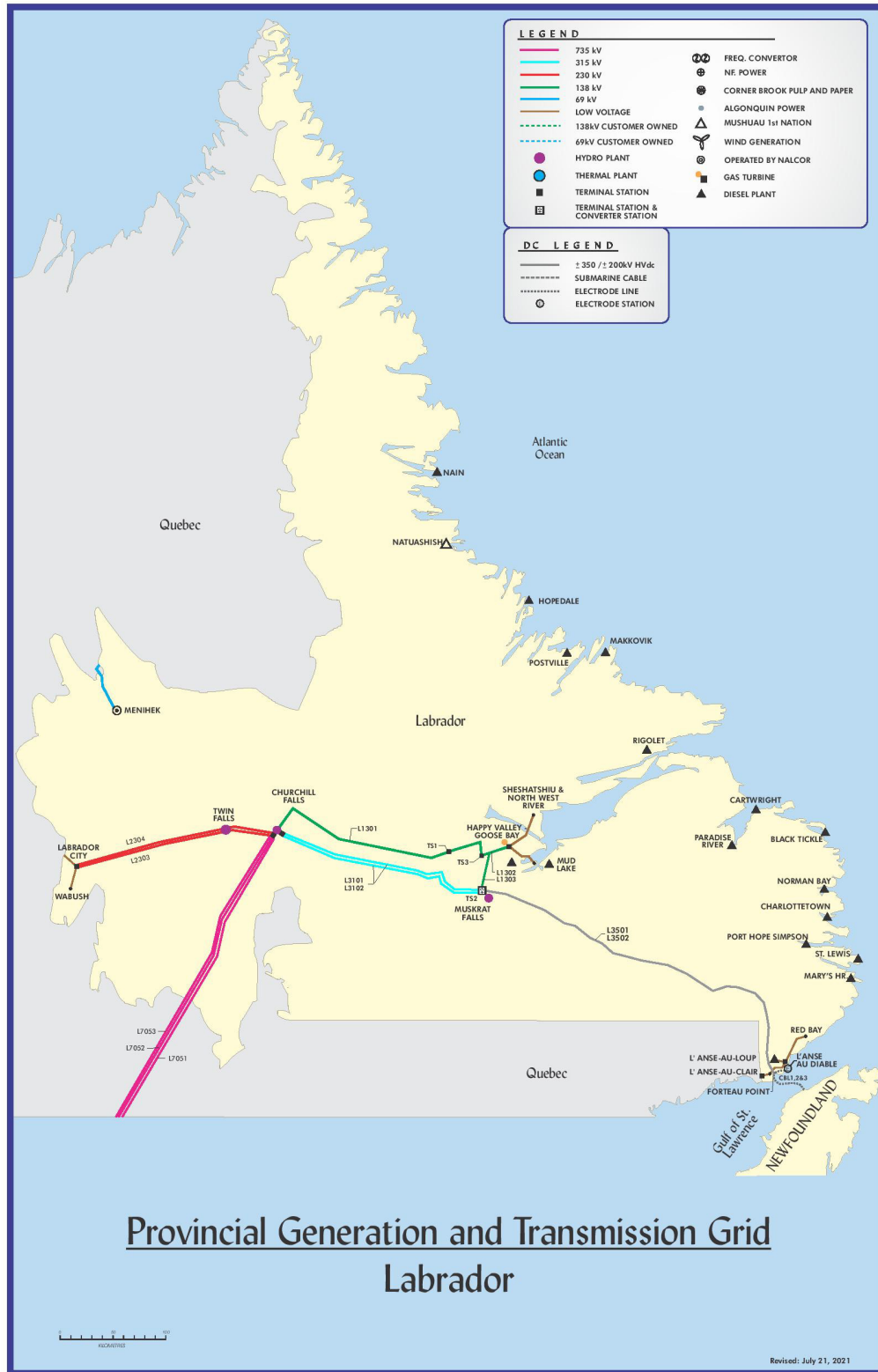
Figure 2: Labrador Interconnected System
