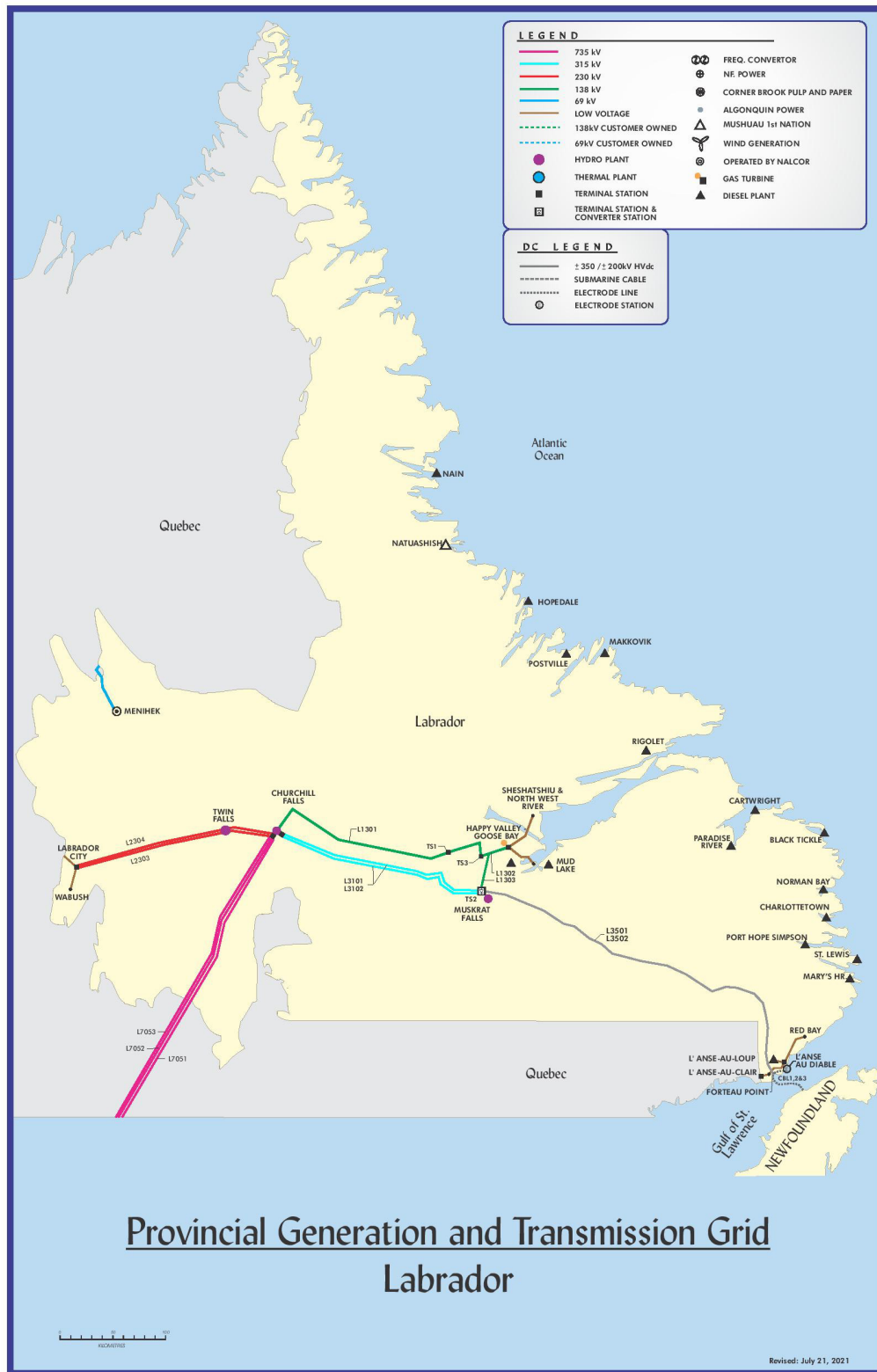
Figure 2: Labrador Interconnected System
